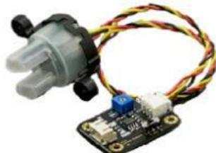
The turbidity sensor measures how cloudy or clear water is. It checks this by using light, depend on the p\_\_\_\_\_ suspended in the liquid. The unite measure is NTU
