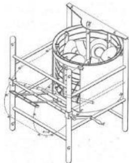
The first dishwasher appeared in 1850 when a man named Joel Houghton made a machine out of wood that splashed water over the dishes inside when you turned a handle.
