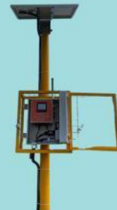
Gambar 5. AWLR (Automatic Water Level Recorder) Sumber: Mertani.co.id
