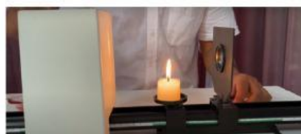
Gambar 2: Set Percobaan Cermin Cekung Sumber: Suparta, Made
