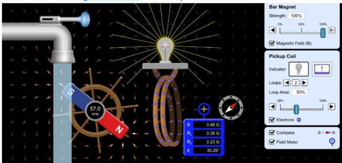
After playing with the simulation, explain how a generator works in three steps
