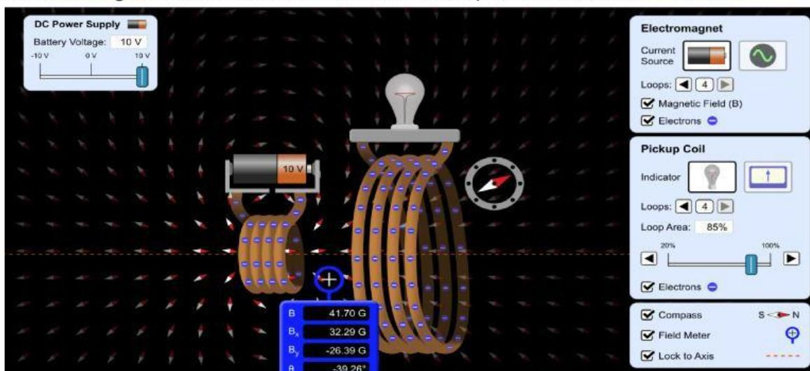
14. The electromagnet on the left is generating a magnetic field that is passing through the secondary loops that attach to the lightbulb on the right. However, it is seen that the bulb does not light up. Use the simulation to figure out how to light up the bulb and then pick the statement that best explains why the bulb did not light up when set up as shown.
