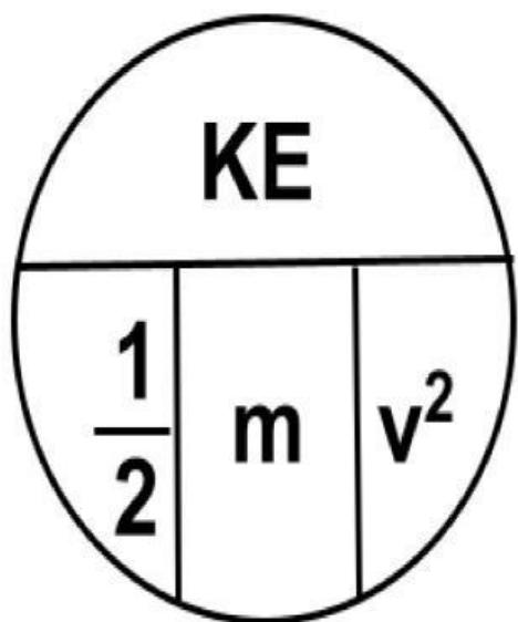
4. A 50 kg mass is moving at a speed of 5 m/s on a flat road. What is its kinetic energy?
