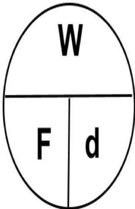
10. A **50 Newton rightward force** displaces an object **4 meters to the right**. What is the amount of work done on the object?
