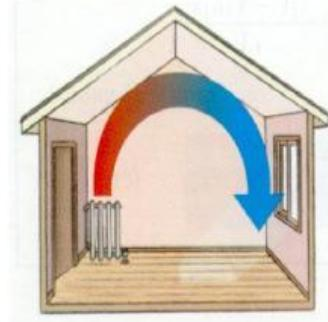
Heated air rises, cools, then falls. Air near heater is replaced by cooler air, and the cycle repeats.
