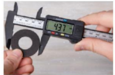
Figure 2.17 Measuring diameter using a pair of digital calipers
