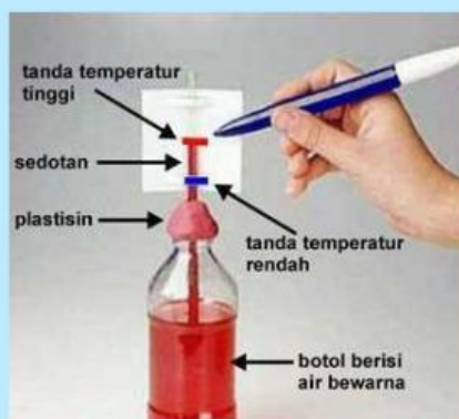
Gambar Termometer Sederhana Sumber : https://www.brainly.com
