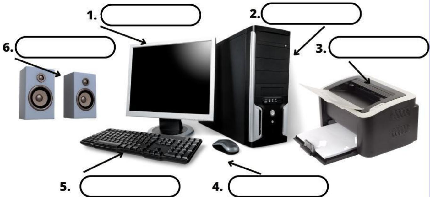
HELP BOX: keyboard - printer - speakers - monitor - mouse - CPU
