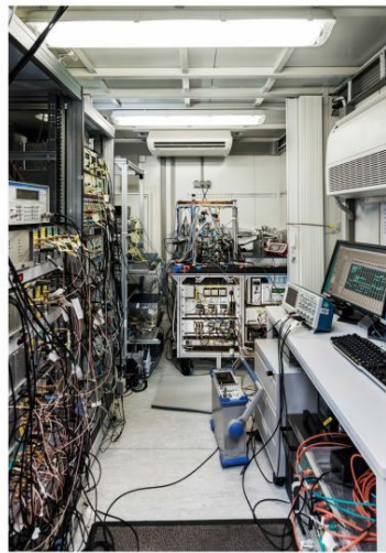
Pictured: Inside view into the trailer with the transportable optical atomic clock.
