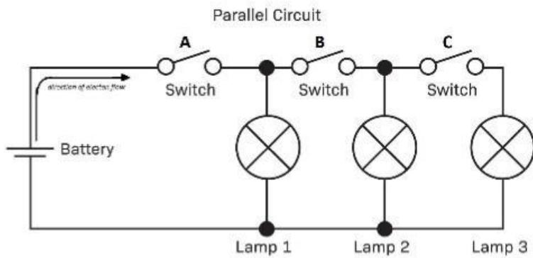
In order for just Lamp 3 to be off which switches should be opened and which should be closed?
