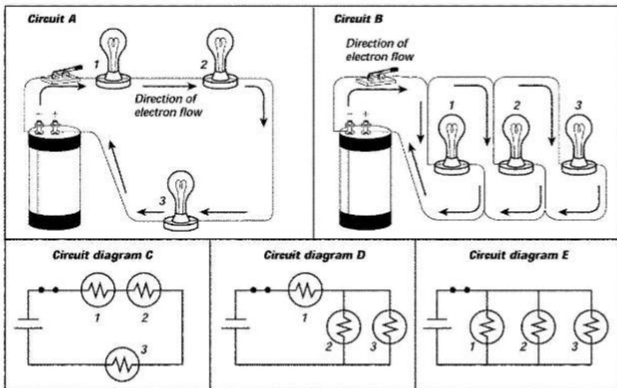
Match the Circuit A and Circuit B with the correct Circuit diagram C, D, or E
