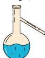
A method of separating mixtures based on differences in their volatilities in a boiling liquid mixture.
