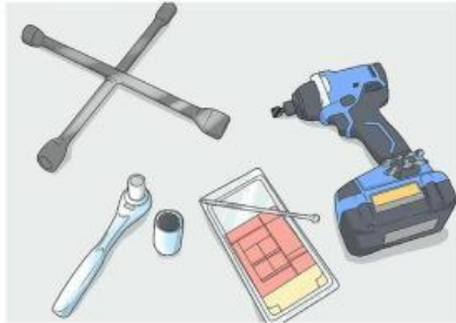
STEP 1: Use the appropriate tool to loosen the lug nuts
