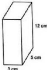
$$\begin{aligned}\text{Volume} &= p \times l \times t \\ V &= 3 \text{ cm} \times 5 \text{ cm} \times 12 \text{ cm} \\ V &= 180 \text{ cm}^3\end{aligned}$$
