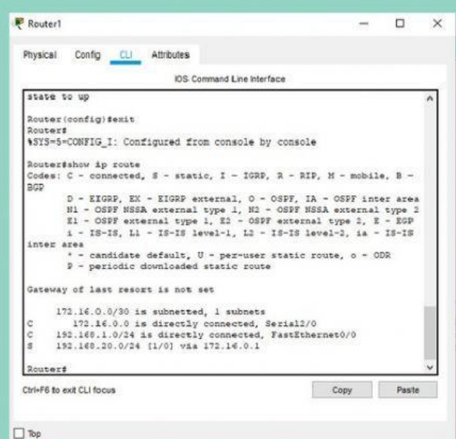
Gambar 13. Pengecekan Tabel Routing Router1
