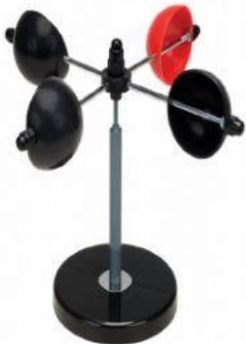
A. It is an instrument that measures wind speed.
