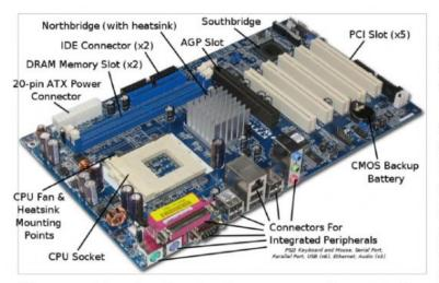
A motherboard is also known as the system board or the main board. The motherboard accommodates the central processing unit (CPU), random access memory (RAM), expansion slots, heat sink and fan assembly, basic input/output (BIOS) chip, system
