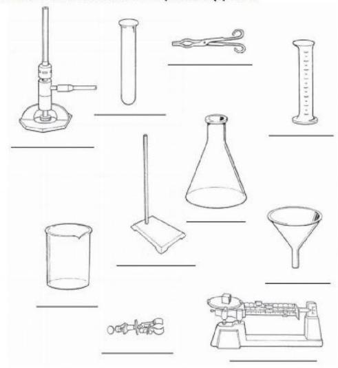
balance Erlenmeyer flask ring stand tongs beaker funnel test tube
