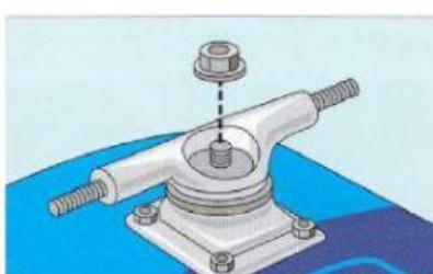
Put the \_\_\_\_\_ on the large bolt. Put the large nut on the large bolt. Tighten the \_\_\_\_\_.
