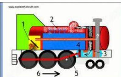
A steam engine is a (1)..... engine that performs mechanical work using steam as its working fluid. The steam engine uses the force produced by steam pressure to push a (2)..... back and forth inside a (3)..... This pushing force is transformed, by a connecting rod and (4)....., into rotational force for work. The term "steam engine" is generally applied only to reciprocating engines as just described, not to the steam turbine.
