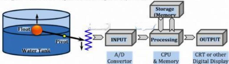
The ..... system above is simple and efficient. However, if more information is needed about the water level, a digital system could be used. ..... are used when data must be stored, used for calculations, or displayed. The input to the system is still a ..... , but an ..... converter is used to convert resistance to ..... The ..... can then manipulate the data as required.
