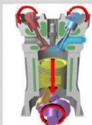
Internal combustion engine intake stroke
