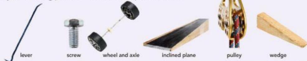
1 A long rigid object that uses a central point to help lift heavy objects.
