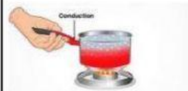
Conductive Heat Transfer
