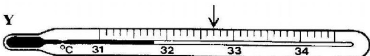
18) Write down the reading to which each arrow points in these diagrams.
