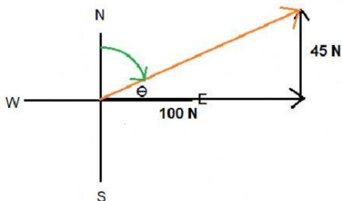
To determine the green angle you need to go all the way to the  $90^\circ$  and then subtract  $\Theta$
