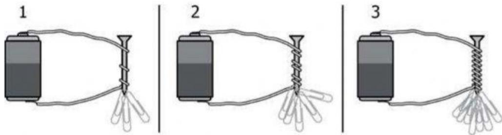
58. A student did an experiment to test the strength of electromagnets. What conclusion could he draw from this experiment?
