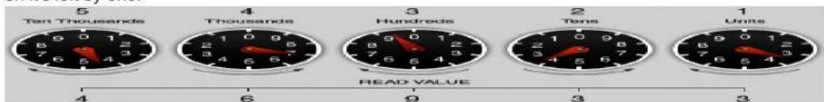
Finding the difference between the present reading and the previous reading of the meter will give the number of kilowatt-hour (kWh) used.
