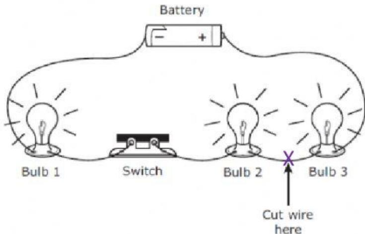
The diagram shows a series circuit with three lit bulbs. How many of the bulbs will remain lit if the wire is cut at the point shown by the arrow?
