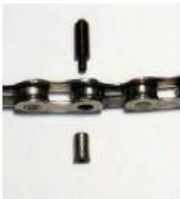
12. A rivet that joins two links on a bicycle chain.
