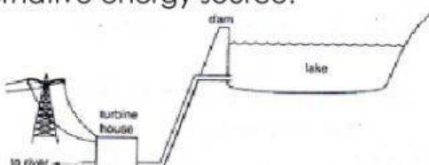
a) Describe how electricity is generated using the energy source shown in figure above. [2]
