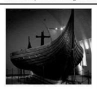
The Gokstand ship was a Viking ship. It was found buried in a farm in Norway, in 1880. It is made of oak and is 24m long x 5m wide.
