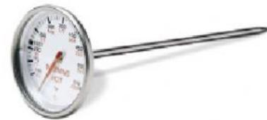
Gambar 4. Termometer bimetal
