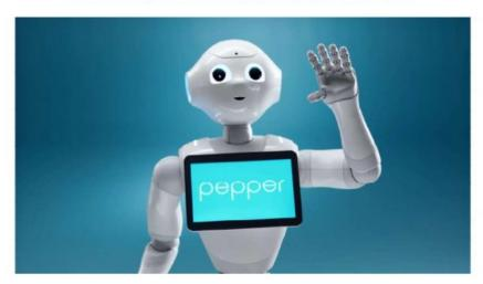
Pepper is a semi-humanoid robot manufactured by SoftBank Robotics (formerly Aldebaran Robotics), designed with the ability to read emotions. It was introduced in a conference on 5 June 2014 and was showcased in SoftBank Mobile phone stores in Japan beginning the next day. Pepper's ability to recognize emotion is based on detection and analysis of facial expressions and voice tones.
