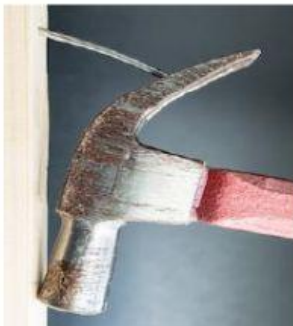
Hammer that removes a nail from the wall.
