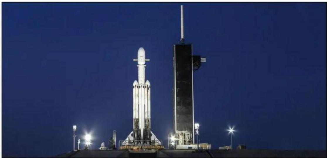
Falcon Heavy is the world's most powerful rocket. It was first launched into space on February 6, 2018 and has been launched two more times since then. Falcon Heavy is a rocket that stands 70 m tall and weighs 1,420,788 kg. Regarding its structure, the first stage has three parts, or cores, each with nine identical rocket engines, making 27 engines in all. Each core is a Falcon 9, an earlier SpaceX rocket. The
