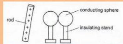
The spheres are then separated and finally the charged rod is removed.
