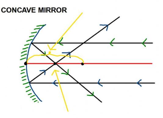
Principle axis Focus Radius of curvature
