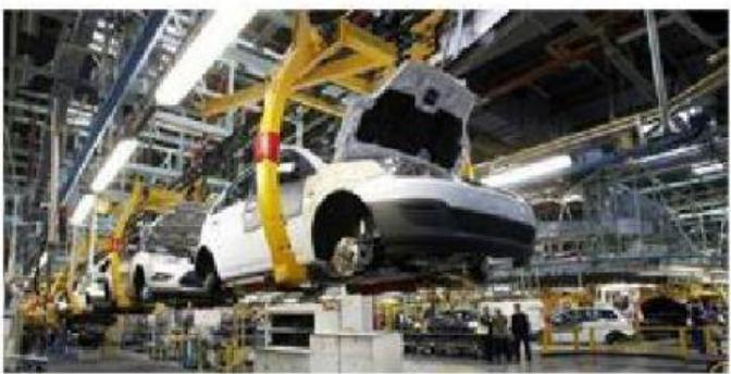
A photograph showing a car being assembled on an overhead conveyor belt in a large industrial factory setting.    | <input type="checkbox"/> | <input type="checkbox"/> |
