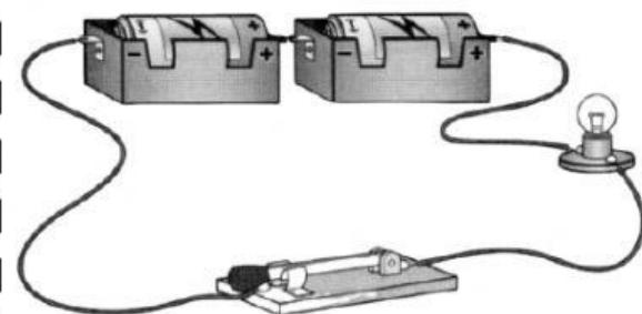
The bulb is not fastened properly into the holder
