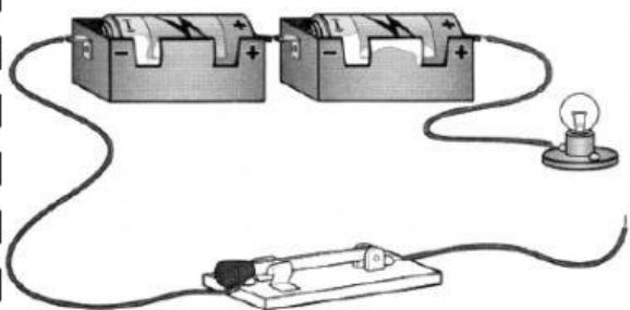
The wire is not connected to the components
