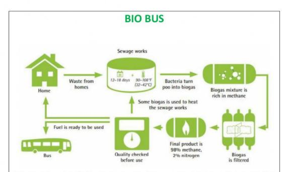
Unlike an ordinary bus, the Bio-Bus has an unusual power supply: human poo. Human waste from sewers can be collected and turned into biomethane, a highly flammable fuel. Because the raw ingredients of biomethane are both plentiful and completely renewable, the Bio-Bus shows us that clean fuel made in this way could one day be used to power our cars, heat our homes, and generate electricity.
