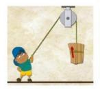
A \_\_\_\_\_\_ is a machine that uses wheels to lift an object. The wheel is attached to high position. A rope is attached to a heavy object and then passed around the wheel.
