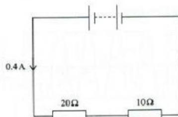
What is the power supplied to the circuit when a current of 0.4 A flows through the  $10\Omega$  and  $20\Omega$  resistors?
