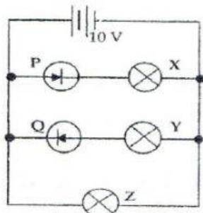
Which component is not working? A. X      B. Y      C. Z      D. P
