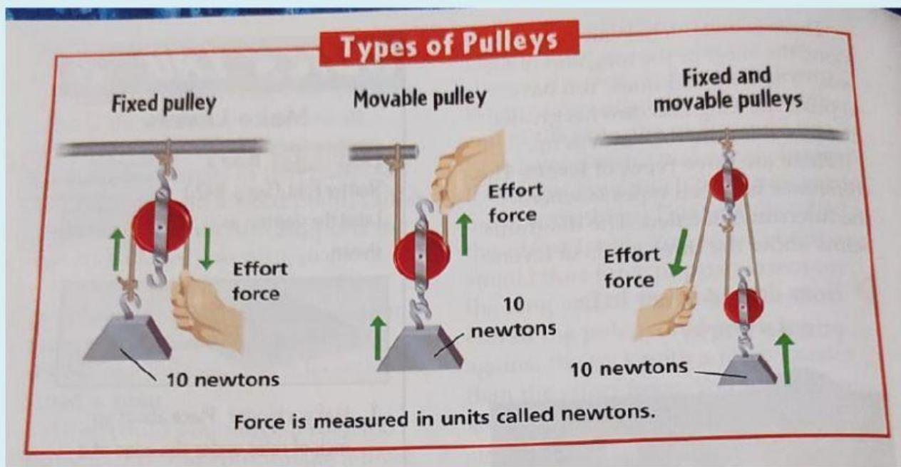
**Name the different types of pulleys.**
