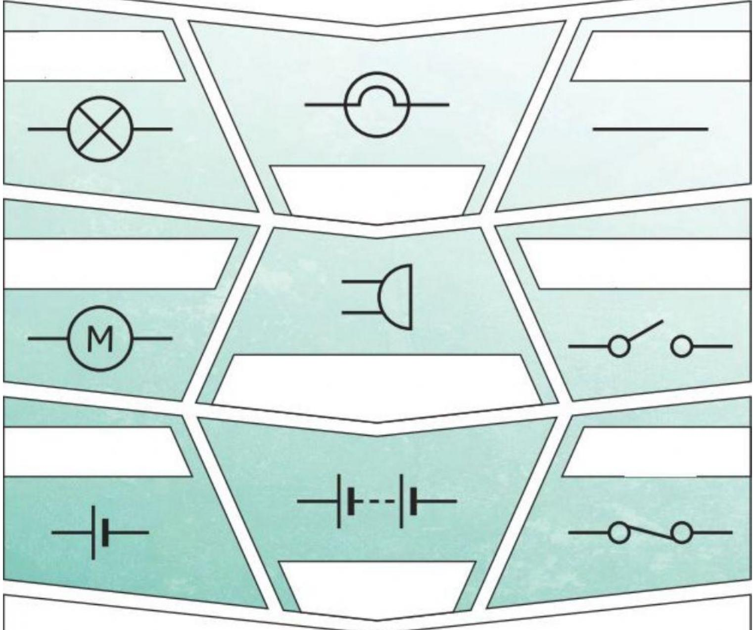
These **symbols** can be used to create electrical **circuit** diagrams.
