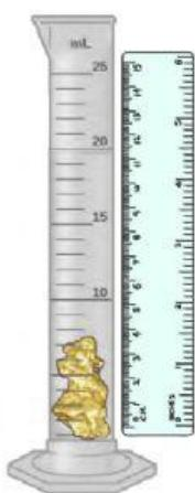
Place water in each graduated cylinder, then put the iron bar in one cylinder, the gold piece in other cylinder and see how much water rises.
