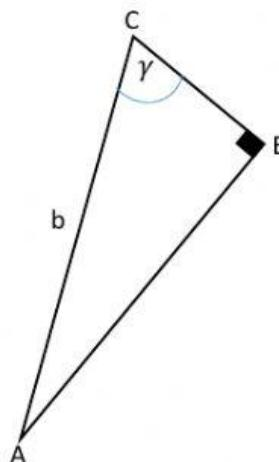
$$\sin \gamma = \frac{\text{sisi depan}}{\text{sisi miring}} = \frac{AE}{AC}$$
