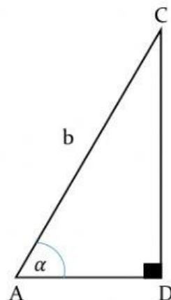
$$\sin \alpha = \frac{\text{sisi depan}}{\text{sisi miring}} = \frac{CD}{AC}$$
