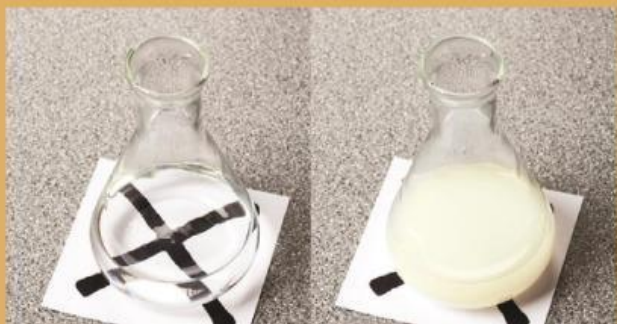
Gambar 1 Percobaan \text{Na}_2\text{S}_2\text{O}_3 + \text{HCl}
